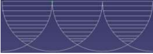
Figure 2. Hatched portion shows the common material to be machined during subsequent feed cycle
