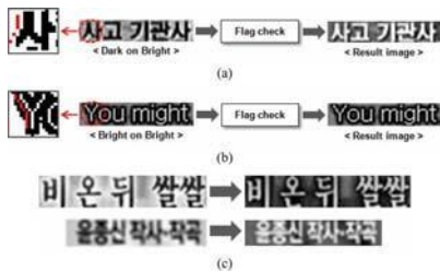
Fig.8. Process of inverting image by the color polarity. (a) Dark text on bright background. (b) Bright text on bright background. (c) Examples of inverted text by “bright_text_flag”.
