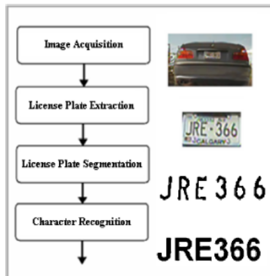
Fig.2. Four Stages of ALPR System
