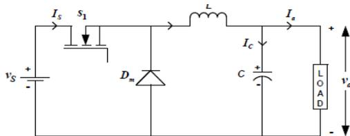
Fig. 3(a) Circuit diagram of buck converter
