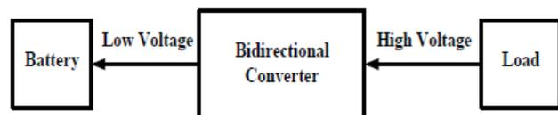
Fig. 2(b) Battery charging mode
