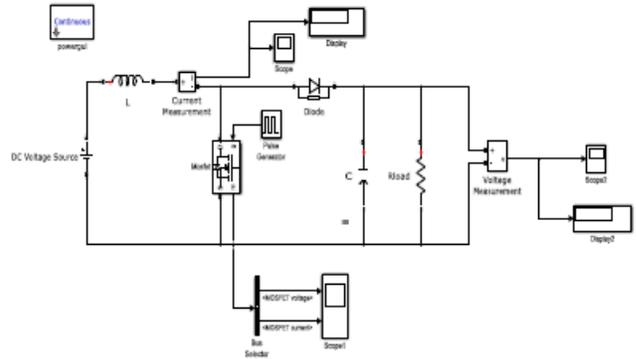
**Fig. 9(a) Simulation model of boost converter**
