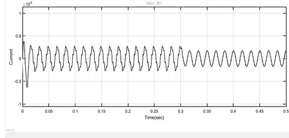
Fig.5. waveform of phase A of load current (without MCR)
