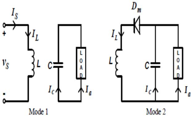
Fig. 5(b) Equivalent circuit of modes of operation
