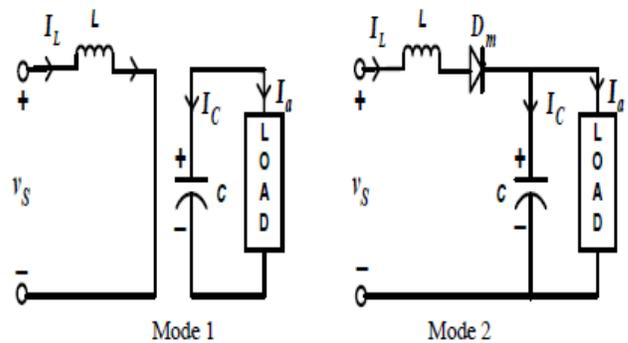
Fig. 4(b) Equivalent circuit of modes of operation
