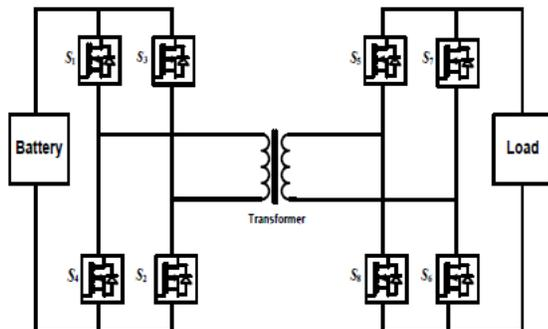
Fig. 1. Isolated DC-DC Converter
