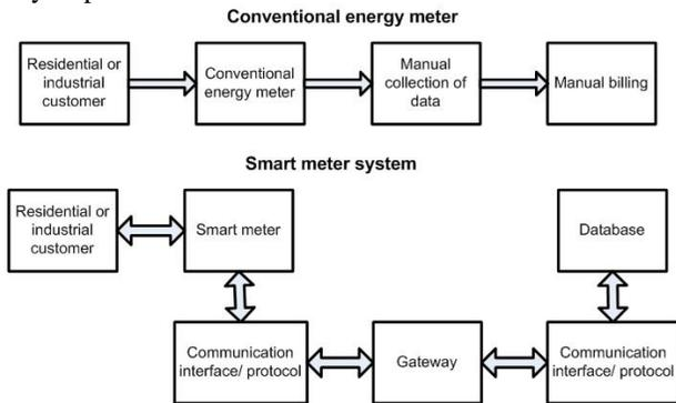
Figure 1. Architectural model of conventional energy meter and smart meter [11].
