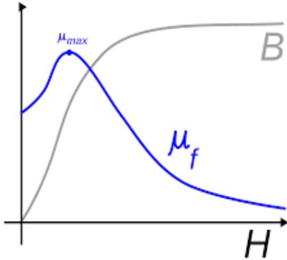
Fig.4. B Vs H &  $\mu$  Vs H curve
