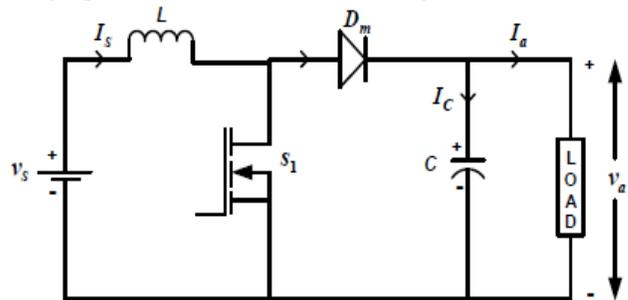
Fig. 4(a) Circuit diagram of boost converter
