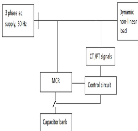
Fig.2. Block diagram of proposed scheme
