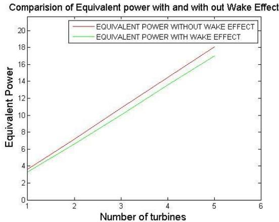
Fig. 6. No. of wind turbine generators vs Equivalent power with and without wake effect
