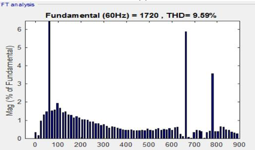
Fig.6. FFT analysis (a) 5th and 7th (b) 11th and 13th
