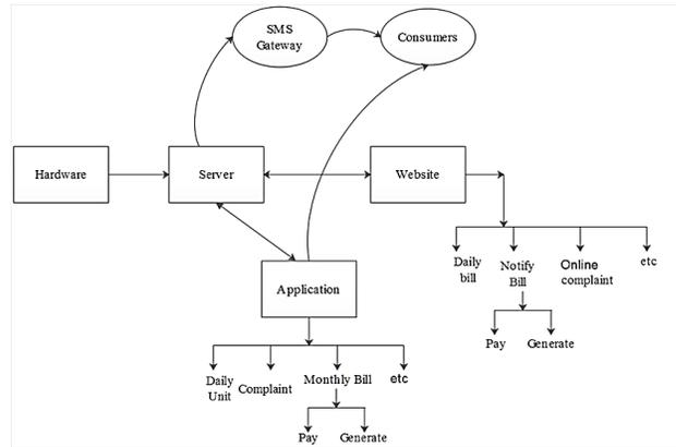
**Fig. 2. Operational Procedure of Smart Grid AMI network**
