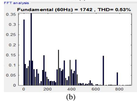
Fig.8. FFT with MCR
