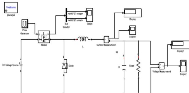
**Fig. 8(a) Simulation model of buck converter**
