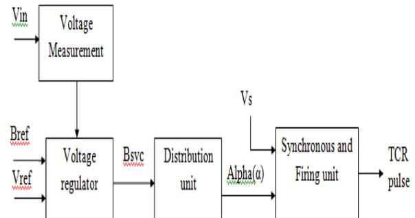
Fig.6. Control scheme for TCR-FC
