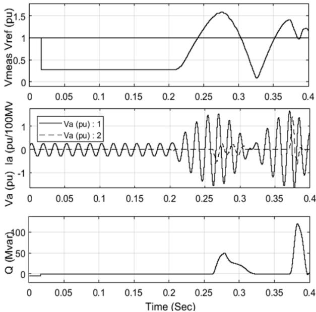
Fig.13. TCR current and voltage
