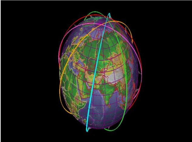
*Fig. 5. Graphical illustration of the out of plane phasing of the designed satellite constellation*
