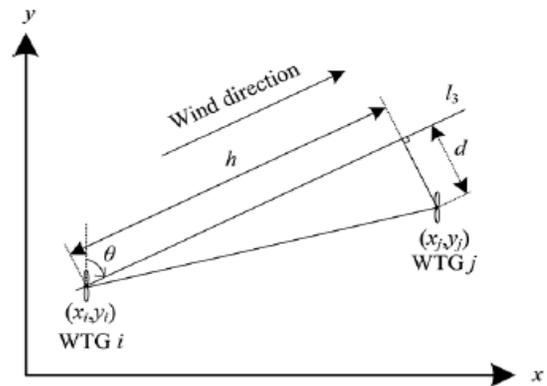
Fig. 3. Horizontal and Deviating distances of two WTGs
