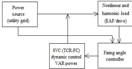
Fig.1. Block diagram of proposed scheme
