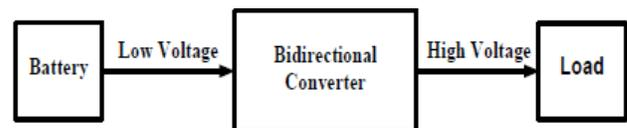
Fig. 2(a) Battery discharging mode
