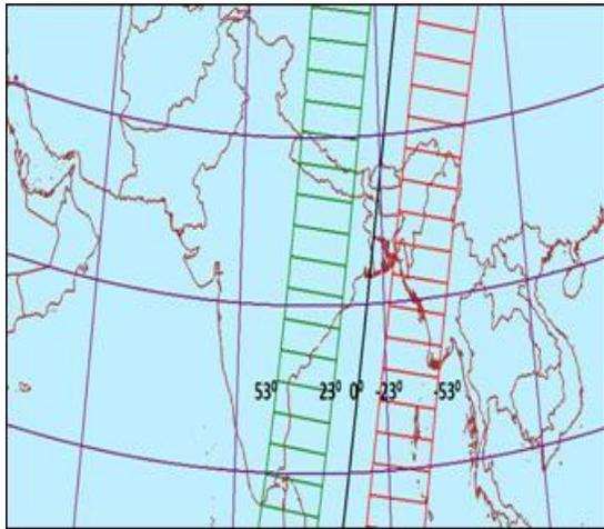
Fig. 2. Satellite ground trace and maximum roll tilt area coverage during a descending pass
