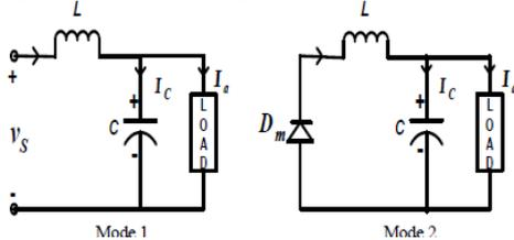
Fig. 3(b) Equivalent circuit of modes of operation
