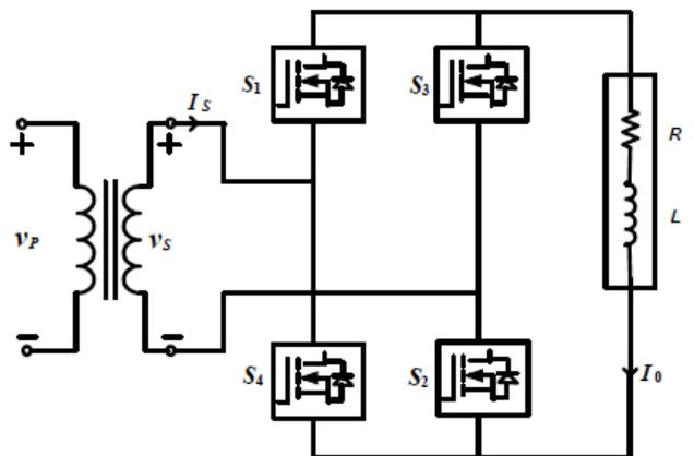
Fig. 7. Single-phase full bridge rectifier
