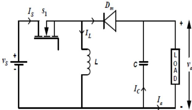
Fig. 5(a) Circuit diagram of buck-boost converter
