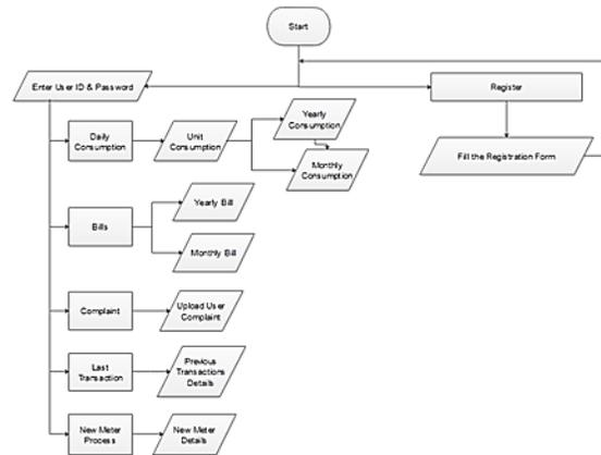
**Fig 3: Data flow diagram of mobile application module**
