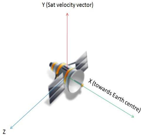
Fig. 1. Satellite Reference frame
