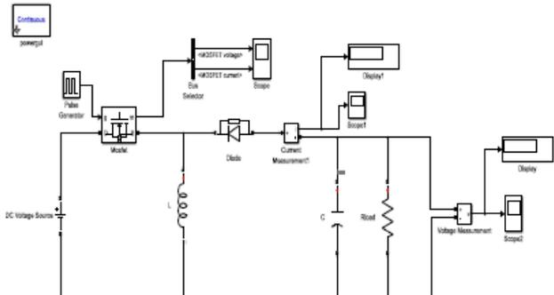
**Fig. 10(a) Simulation model of buck-boost converter**
