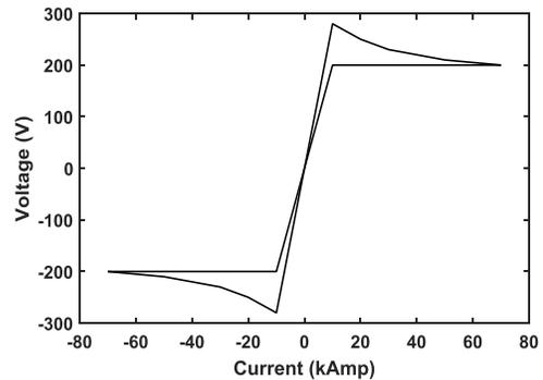
Fig.3. Dynamic V-I characteristic of arc furnace
