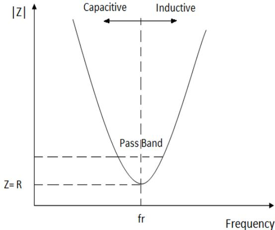
Fig.1. Single Tuned harmonic filter |Z| vs Freq
