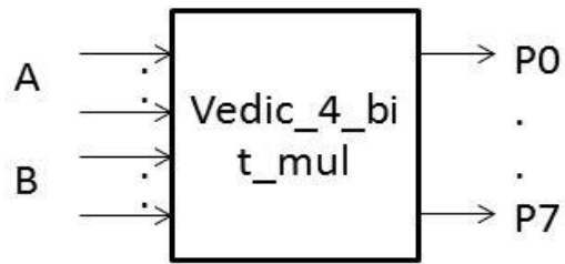
Figure 3: Block Diagram of a 4 bit Vedic Multiplication
