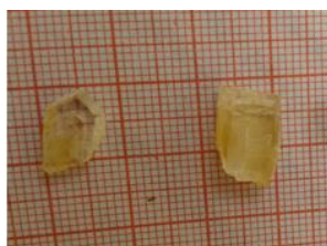
Photograph of the grown crystals of tetrakis-thiourea trichloroacetic acid
