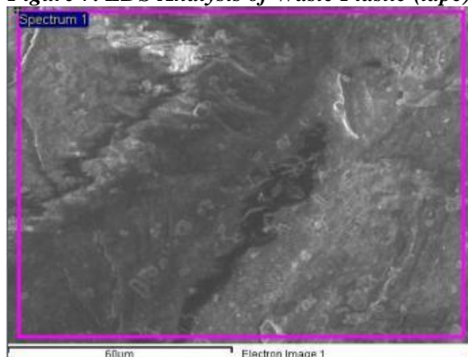
Figure 7. EDS Analysis of Waste Plastic (ldpe)
