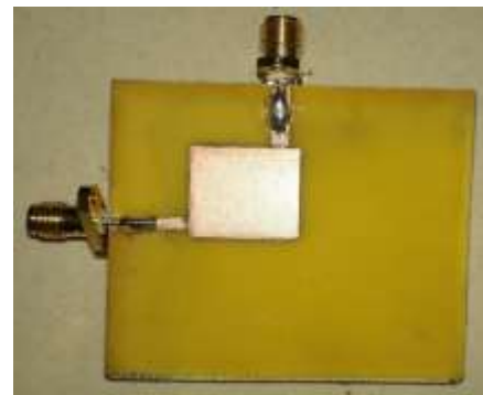
Fig.2. Hardware implementation of antenna
