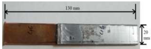
Figure 3. Specimen for tensile shear strength test
