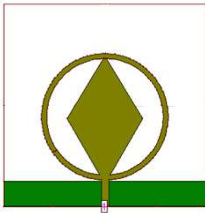
Fig. 1: Annular Ring combind with Diamond Patch
