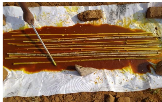
Fig 5. Bamboo Splints in Chemical Solution
