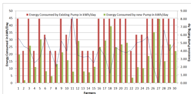
Fig.3: Comparison of energy consumed with excess pump capacities
