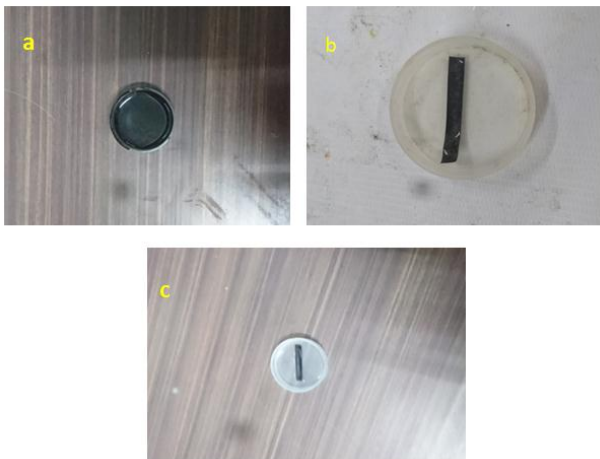
Fig.2. (a is the Viscous solution of GO/PANI, b is s the coated film, and c is the film dipped in 1.5N lithium chloride solution for cat ion exchange process).
