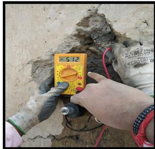
Fig No.-3.Half cell test
