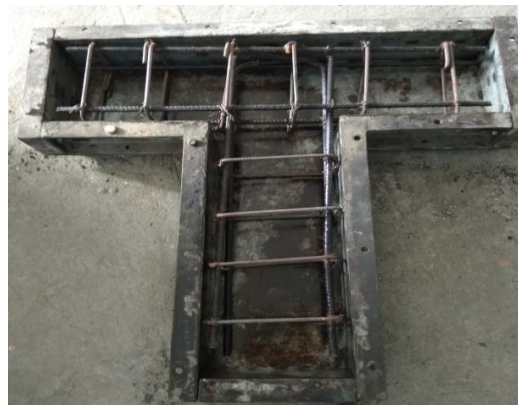
Fig-03-Reinforcement details of beam column joint
