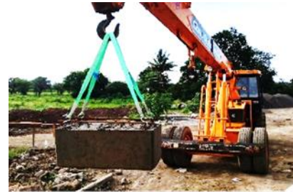
Fig. 5.1.2: Remove block from mold
