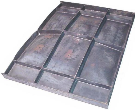
Figure (7) Failure of Stiffened Plate in experiment
