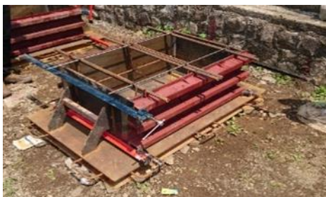
Fig.5.1.1: Steel mold for block casting
