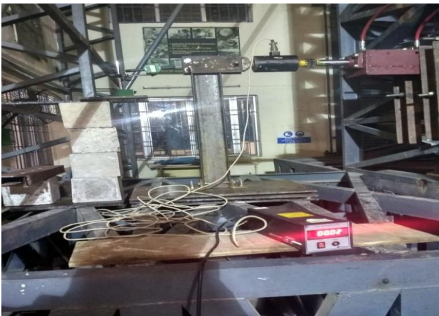
Fig.5 Testing arrangement for lateral loading
