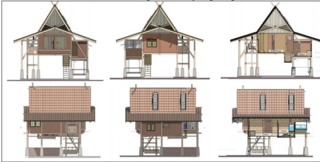
Figure 6. Front, back, and side elevation of flood-friendly in Cieunteung
