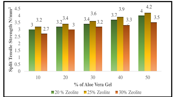
GRAPH. 1.6: SPLIT TENSILE STRENGTH OF CONCRETE WITH AND WITHOUT ZEOLITE AND ALOE VERA
