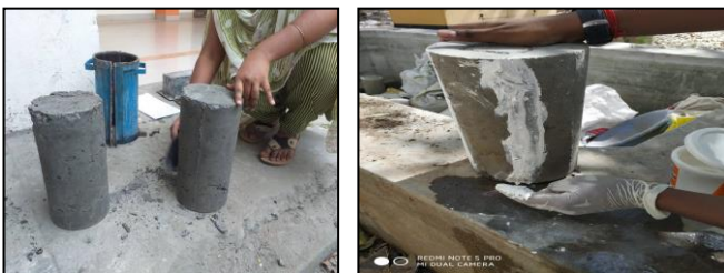
Figure 2 Casting and repairing of cylinders
