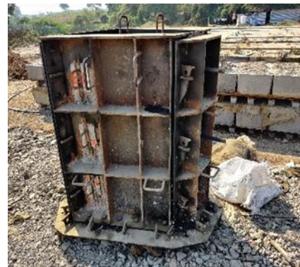
Fig.5.1.4 Steel mold for socket casting
