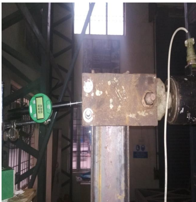
Fig. 6 Position of Dial Gauge
