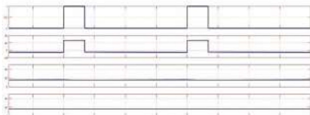
Fig. 10. From top to bottom: (a)Gate signal, (b) Inductor voltage and capacitor voltage Cx and Cy
