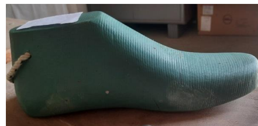
Fig.6 Development of shoe last according to proportional measurements
