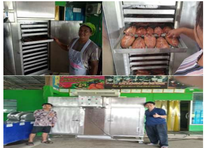
Figure 3 The heat pump dryer for drying single sun-dried snake-head fish.
