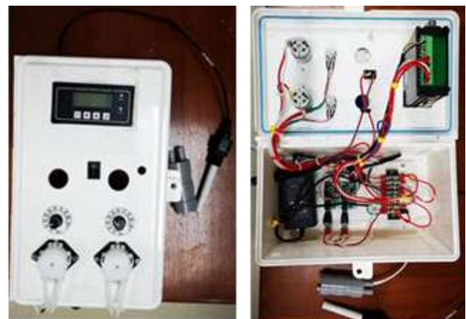
Figure 6: Automatic solution mixing equipment
