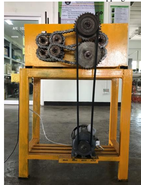
Fig. 2 Power unit and power transmission of the bamboo stripping machine
