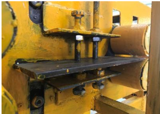
Fig. 5 Blade number 1 of the bamboo stripping machine
