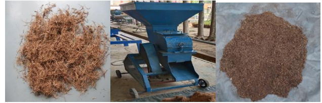
Fig 3.1 Hammer mill machine to crush oil palm empty fruit bunching fibers
