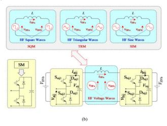
Fig.1. (b) Dual-active phase-shift principle of SST
