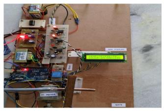
Fig 4.4 Temperature of the person entering and count of persons present in the room are displayed on LCD
