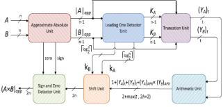
Fig. 2.Proposed approximate signed multiplier block diagram.
