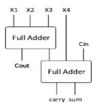
Figure. 3. Structure of the 4:2 compressor.
