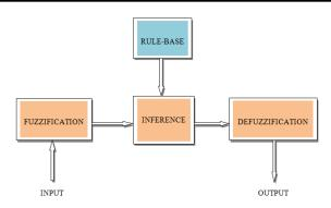
Fig.2. Block diagram of fuzzy logic control
