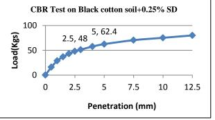
Figure 2: CBR Test on Black cotton soil+0.25% SD
