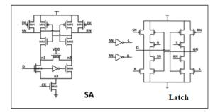
Fig.7 Circuit diagram of Nikolic Flipflop.
