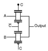
Fig.15 2: 1 mux using Transmission gates.
