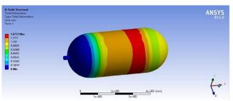
Fig. 5. Static Structural Deformation of Steels515-gr70
