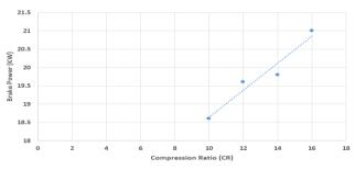
Figure 14. CR versus Brake Power
