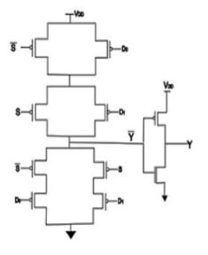
Fig.16 CMOS Logic Using 2:1 mux.
