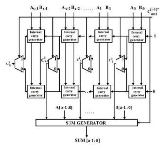
Fig 4: proposed inexact speculative adder
