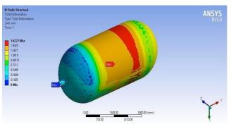
Fig. 17. Static Structural Deformation of Steel-s515gr70 and Epoxy Carbon
