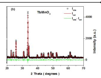
Figure 1: (a) XRD of TbMnO<sub>3</sub> sample. (b) Rietveld refinement pattern of TbMnO<sub>3</sub> samples.
