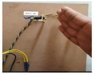
Fig 4.7 when a person exits from exit entrance the IR sensors are interrupted and the count of persons available is decreased by one.
