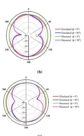
(c) Fig. 11. Radiation patterns at a) 2.9 GHz b) 5.5 GHz c) 7.5 GHz
