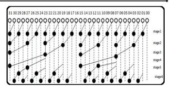
Fig.8 Carry generation of an 32-bit Brent-Kung adder
