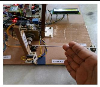
Fig 4.3 When IR sensor detects a person at the entrance of the room.
