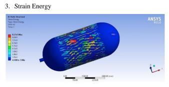
Fig. 19. Static Structural Strain Energy of Steel-s515gr70 and Epoxy Carbon
