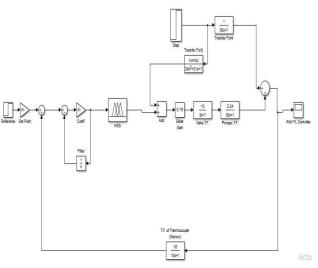
Fig.9. Simulink model of HES with FLC
