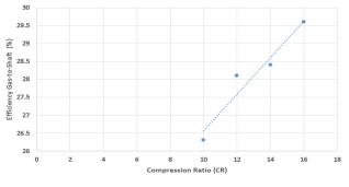
Figure 7. CR versus Efficiency Gas-to-Shaft
