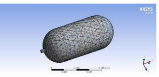
Fig. 3. FE Tetra-Mesh of Pressure Vessel in Ansys Workbench
