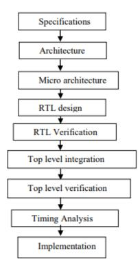
Fig: Flow chart of the VLSI design
