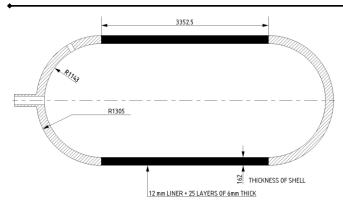
Fig. 17. Line Diagram of the Multi-layered Composite Pressure Vessel
