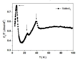
Figure 2: Variation of Cp/T with temperature
