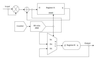
Figure 3: proposed power detector architecture
