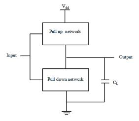
Fig.4(a) Basic CMOS circuit structure
