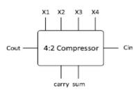
Fig.2. 4:2 compressor block diagram.
