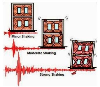
Fig 1: Performance objectives under different intensities of earthquake shaking (Murty 2005)
