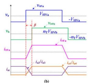
Fig.2. (a) Voltage waveform (b).Current waveform for Square High-Frequency-Link Modulation
