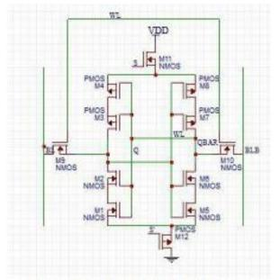
Fig4:12T SRAM -Cell schematic
