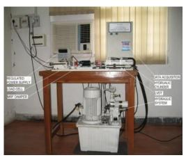
Fig.4: Experimental setup of MRF damper (Courtesy
