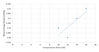
Figure 6. CR versus Mixture Energy Density
