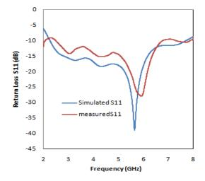
Fig. 10. Simulated and measured return loss of the proposed antenna
