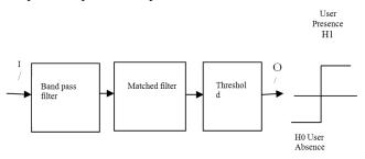
Fig1: Matched Filter Detector
