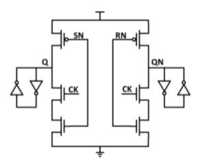
Fig.8 Circuit diagram of Kim's latch.
