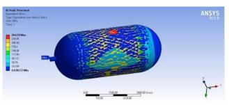
Fig. 18. Static Structural Von-Mises stress of Steel-s515gr70 and Epoxy Carbon
