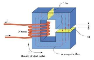
Fig 1: circuit details of magnet
