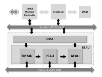
Fig. 1. DLAU accelerator architecture
