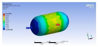
Fig. 12. Static Structural Von-Mises stress of Epoxy e-Glass
