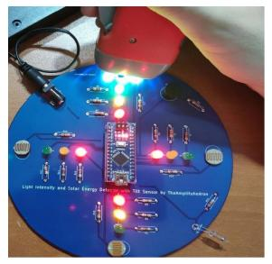
Fig.12.Testing of performance levels Low (Red), Moderate (Yellow) High (Green) in each direction
