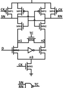
Fig.11 Circuit diagram of Jeong SAFF
