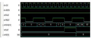
Figure 12: Simulation result of slave for single read data operation
