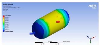
Fig. 6. Static Structural Von-Mises stress of Steels515gr70 3. Strain Energy
