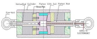
Fig. 2: Sectional view of the developed device (Courtesy [8])
