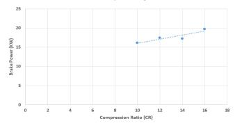
Figure 5. CR versus Brake Power
