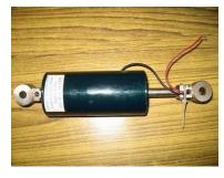
Fig.3: MRF Damper
