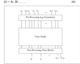
Fig.6 Block Diagram of Parallel prefix addition.
