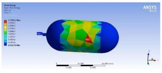
Fig. 13. Static Structural Strain Energy of Epoxy e-Glass
