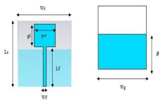
Fig. 2 .Geometry of square patch antenna with Partial Ground Plane (a) front view (b) back view
