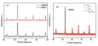
Figure 1. (a) X-Ray diffraction patterns of LBMO and Zn doped LBMO. (b) Rietveld refinement profile of LBMO.
