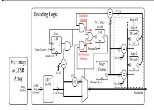
**Fig.5.**Logic for decoding the binary representation of the LFSR counter state order with multiple stages. Each stage is decoded one at a time in the correct order.
