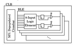
Fig.6. Hybrid CLB with a 50% depopulated intra-CLB crossbar depicting BLE internals for a fracturable (two optional registers and two outputs) architecture.
