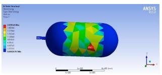
Fig. 7. Static Structural Strain Energy of Steels515-gr70
