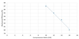
Figure 9. CR versus Mechanical Efficiency
