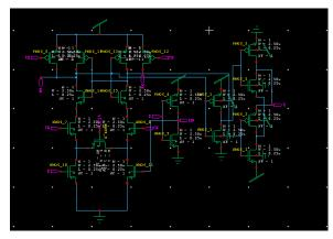
Fig. 19 schematic diagram of proposed SAFF using GDI based latch.
