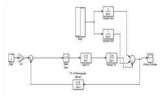
Fig.3. Simulink model of heat exchanger system without controller
