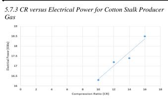
Figure 13. CR versus Electrical Power
