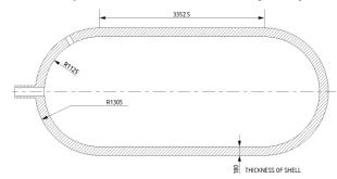
Fig. 1. Line Diagram of the Pressure Vessel
