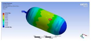
Fig. 9. Static Structural Von-Mises stress of Epoxy s-Glass
