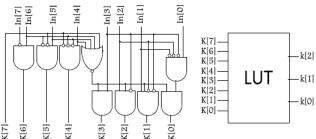
Fig.3. Schematic of the Leading-One Detector Unit for 8-bit input operands.
