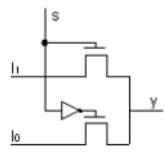
Fig.17 2:1 mux using pass transistor Logic.
