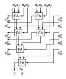
Fig. 4. Structure of the 8:2 compressor.
