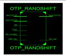
Fig 8:RTL Schematic of OTP Rand shift using magnitude comparator
