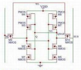
Fig3:10T SRAM -Cell schematic
