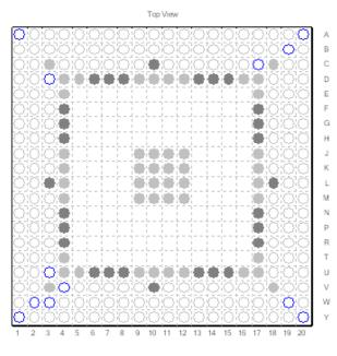
Fig. 10: Pin layout of the implemented design for the targeted FPGA
