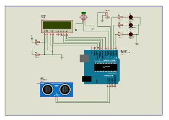
The open and close automatically water gate operation is illustrated in block diagram system (Figure 2). The diagram contains several parts, that is, water level detected by the ultrasonic sensor, input data from ultrasonic sensor to Arduino, Arduino set servo motion, the servo for moving the water gate (the door aquarium), and the ultrasonic sensor for making feedback to Arduino. If the water level is low so the door would close.
