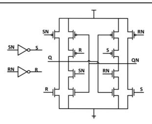
Fig.10 Circuit diagram of strollo's Latch
