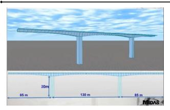
Figure 2. Dimensional Properties of Bridge
