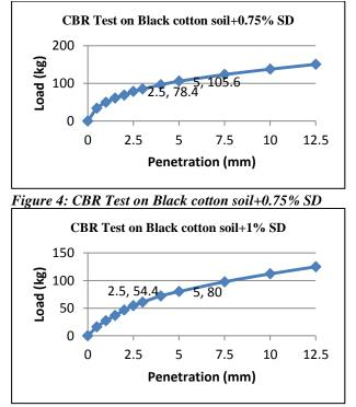
Figure 5: CBR Test on Black cotton soil+1% SD
