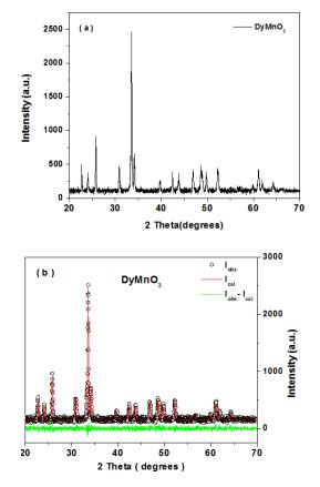
Figure 1: (a) XRD of DyMnO3 sample. (b) Rietveld refinement pattern of DyMnO3 samples.
