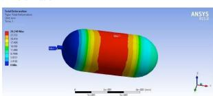
Fig. 11. Static Structural Deformation of Epoxy e-Glass
