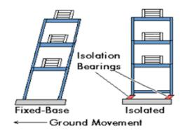
Fig.4: Building with fixed base and with base isolation [9].
