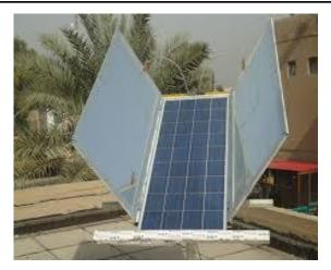
Fig.1: Effect of Angle Orientation of Flat Mirror Concentrator on Solar Panel System Output.
