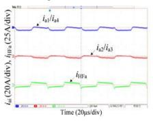
Fig.9 gives arm current waveforms for square modulations in the SST. It is confirmed that all the arm currents are also high-frequency ac waves with 20-kHz frequency that are similar to HF link currents, however, there is a dc bias. The arms 1 and 4 have the same current, the arms 2 and 3 have the same current, the arms 1/4 and 2/3 are having the complementary currents.
