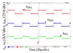
Fig.8. HF link voltage and current waveforms in SST
