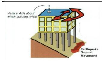
Fig. 2: Torsional behavior of building on sloping ground [8].
