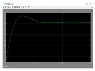
Fig.6. Response of heat exchanger system with PID controller
