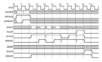
Figure 1: Write address and data burst.
