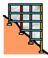
Fig. 1: Building on sloping ground have long and short column which may twist during earthquake [8].
