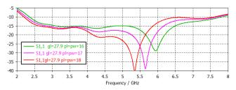
Fig. 4. Parametric plot of Return Loss for gl=27.9 for different values of pl and pw
