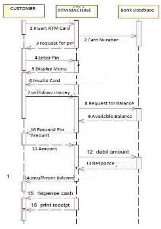
Fig 1. Sequence diagram for ATM Withdraw
