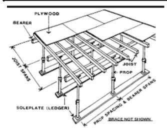
Figure 4: Diagram of the formwork (Source: Collected by the researcher)
