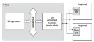
**Fig: Processor-SPI Interaction**
