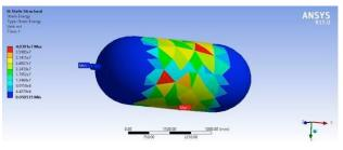
Fig. 10. Static Structural Strain Energy of Epoxy s-Glass
