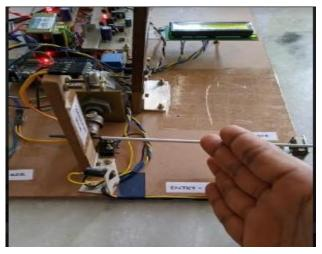
Fig 4.6 Displays the gate closure when a person wants to enter when the limit reaches the maximum count set.
