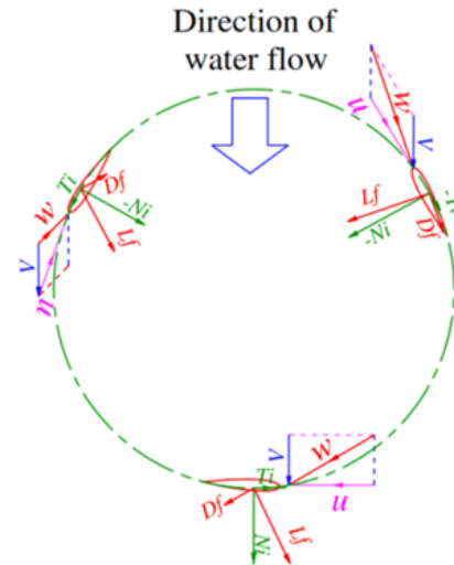
Fig. 4. The velocity and force conditions are various orientation of vanes [12]
