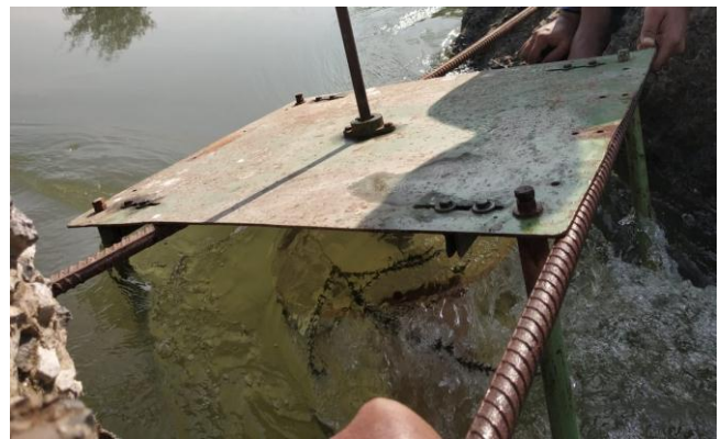
Fig. 8. Turbine model at Inclination angle in a canal
