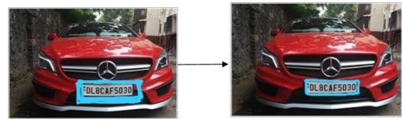
Figure 4: Working of non_max_suppression_fast_function
