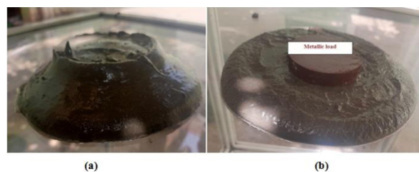
Fig2: Spreading (a) Without Load and (b) Under Load
